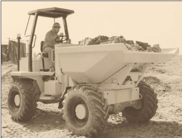
Figure 7 Site dumper with ROPS
